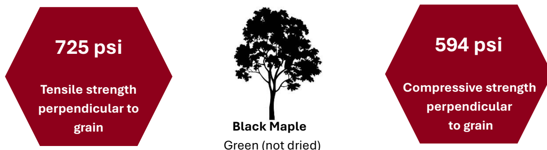
Figure 15. Mechanical strength of maple wood
